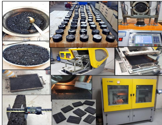
Figure 2: Marshall and slabs compaction and testing. Source: Own elaboration.
