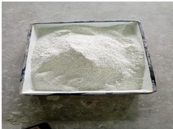
Figure 4: Kota Stone Slurry. Source: Own elaboration.
