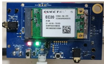
Figure 8: Cellular module for Gateway link. Source: Prepared by the authors.
