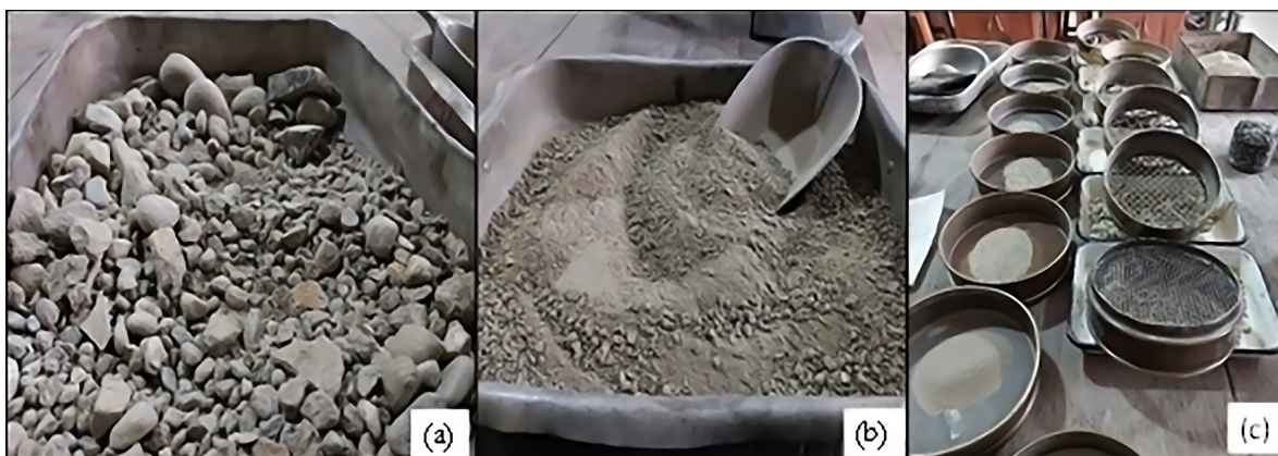
Figure 1. Sieve analysis process for gradation determination. (a) Aggregate sample prior to sieving; (b) Sample passing sieve No. 4 for mixture design; (c) Sieves employed for the analysis.
