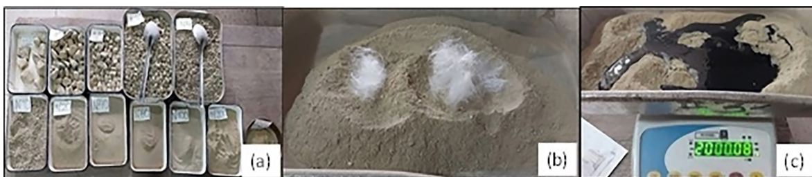
Figure 2. Process of preparing modified asphalt mixtures with microfiber reinforcement. (a) Aggregate separated for gradation construction; (b) Aggregate combined with microfiber; (c) Aggregate, microfiber, and liquid asphalt.
