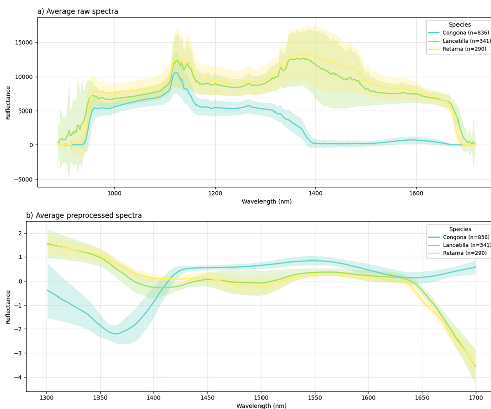
Figure 2. Relative absorbance spectra of the three studied species: Peperomia inaequalifolia , Alternanthera sp., and Teline monspessulana . (a) Raw spectra. (b) Cropped spectra (1300–1700 nm) preprocessed with Savitzky–Golay derivative and SNV.
