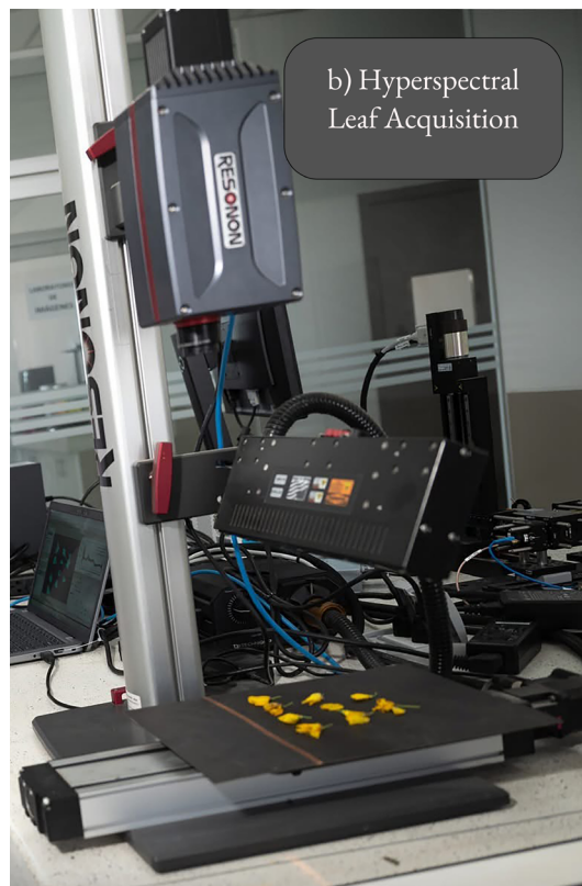
Figure 1. a) Workflow for medicinal plant classification using machine learning; b) Spectral acquisition by hyperspectral imaging.
